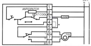
\*LINK 4 & 5 FOR FAN CONTINUOUS,3 & 5 FOR FAN AUTOMATIC (CYCLED)
