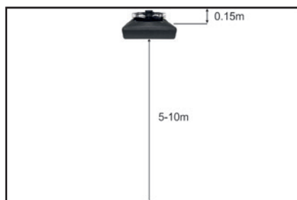
Montering i loft
